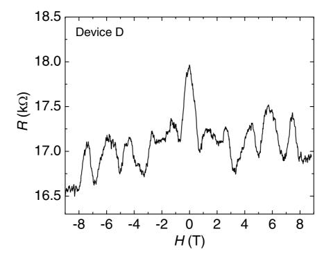
**Figure S5. Magnetoresistance curve of device D**. The magnetoresistance curve of device D was measured at 2 K. The width and length of the nanowire are 80 nm and 500 nm, respectively. The robustness of AB oscillation at high field is evident.
