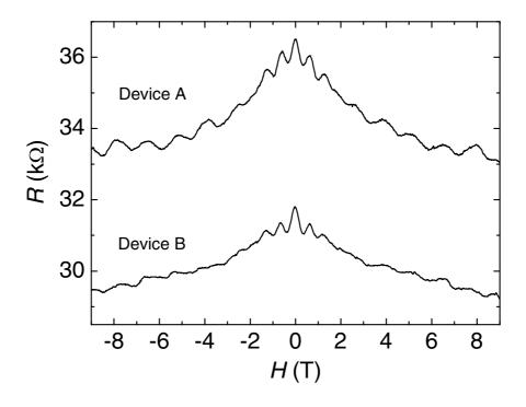
**Figure S2. Comparison of the magnetoresistance (MR) of the devices A and B.** The MR curves were measured for devices A and B fabricated on a single nanowire. Although there exist about 10% of difference in the two-probe resistances, two devices exhibited almost identical MR features.
