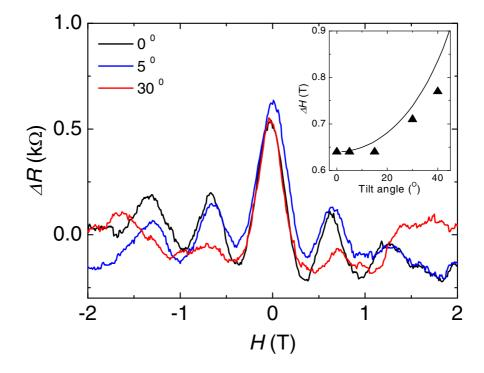
Figure S3. Angle-dependence of the AAS oscillation. The change of the MR curve with the tilt angle  $\theta$  is shown; 0° (black), 5° (blue), and 30° (red). Inset shows the first oscillation period as a function of the tilt angle. The oscillation period fits relatively well to the expected  $1/\cos\theta$ -law (solid line).
