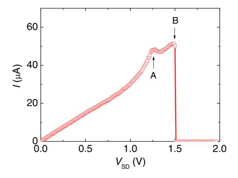
**Figure S4. High bias characteristics of device C**. We have measured high-bias characteristics of the device C. With high-enough bias voltage, abrupt drop of current due to the breakdown of the nanowire was observed. For our devices, two-step breakdown, denoted as A and B, were generally observed. At the point A, the current does not go to zero and the breakdown of the outer shell part is presumed. At the point B, current drops to zero, indicating breakdown of the nanowire core.
