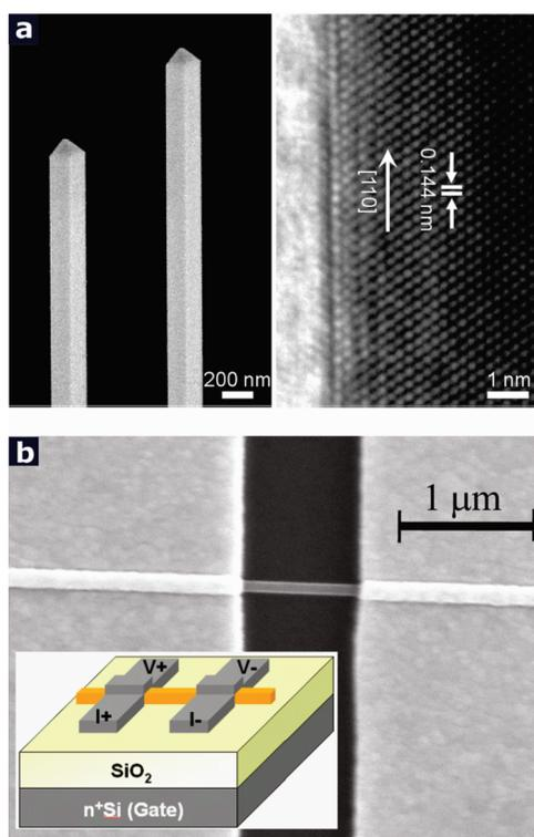
**Figure 1.** (a) Scanning electron micrograph (left) and a high-resolution TEM image (right) of single crystalline Au NWs. (b) SEM image of the Au NW device. Inset: A schematic view of the device and the measurement configuration.
