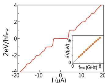
**Figure 4.**  $I$ - $V$  characteristics under a microwave field of frequency  $f_{\text{mw}} = 4.6$  GHz at  $T = 260$  mK.  $V$  was normalized by  $hf_{\text{mw}}/2e$  to make the integer and the half-integer Shapiro steps clearly identifiable. Inset: voltage spacing unit ( $\delta V$ ) between the integer steps versus  $f_{\text{mw}}$ . The solid line is a direct plot of  $hf_{\text{mw}}/2e$  without any adjustable parameters.
