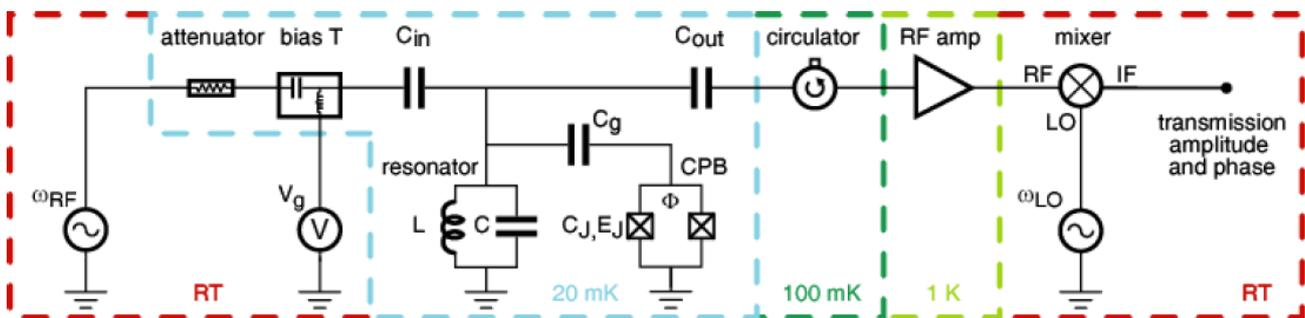
Figure 6 : Superconducting circuit. The dashed coloured zones represent the temperatures zone: RT : Room Temperature, other abbreviation in the glossary.[8]
