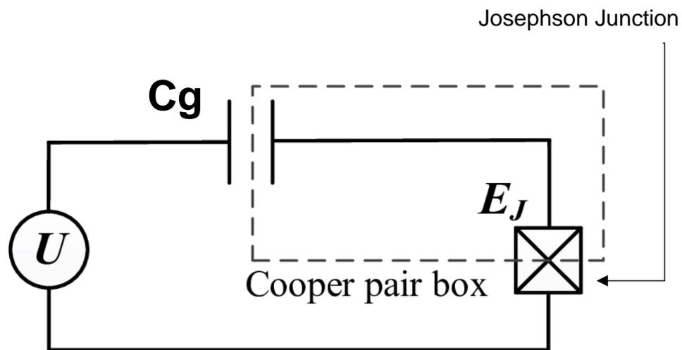
*Figure 3 : Circuit of a charge qubit [adapted from [6] ]*
