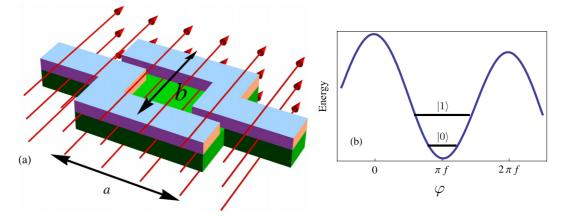
Figure 1. (a) A schematic of a superconducting phase qubit coupled to a torsional resonator. The arrows denote the external magnetic field. (b) A schematic of the energy levels corresponding to the logical basis states  $|0\rangle$  and  $|1\rangle$  of a phase qubit.
