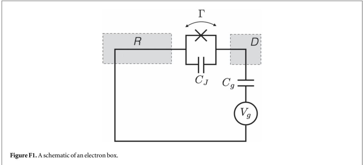
**Figure F1.** A schematic of an electron box.
