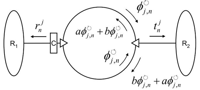
Fig. 2. The schematic picture for the setup of a ring attached to two leads. Two reservoirs are denoted as  $R_1$  and  $R_2$ . Like in Fig. 1, the partial waves are labeled as  $\phi_{j,n}^\ominus$  and  $\phi_{j,n}^\circ$ , where  $j$  represents from which arm the atom enters the junction, namely  $u$  (the upper arm) or  $d$  (the lower arm).
