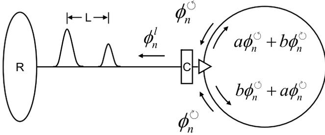
**Fig. 1.** The schematic picture of the setup for a ring attached to a single lead. R and C represent a reservoir and a microcavity, respectively. The partial waves in the ring entering the junction are represented as  $\phi_n^{\odot}$  (clockwise) and  $\phi_n^{\ominus}$  (counter-clockwise), and the waves outgoing along the leads is labeled as  $\phi_n^l$ . In semiclassical description the successively escaping wavepackets are separated with each other by  $L$ .
