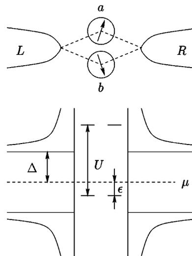
FIG. 1. Upper panel: sketch of the superconductor-double quantum dot-superconductor (*S*-DD-*S*) nanostructure. Lower panel: schematic representation of the quasiparticle energy spectrum in the superconductors and the single-electron levels of the two quantum dots.
