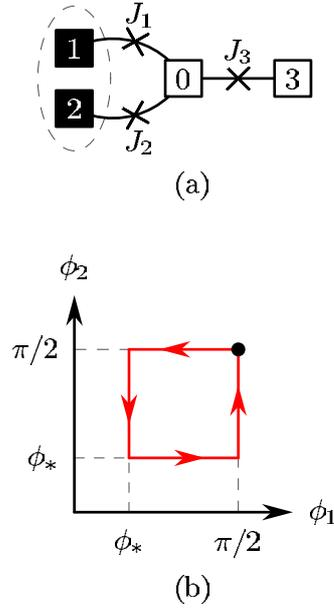
**Figure 5.** (a) Configuration for a rotation around the  $x$ -axis,  $U_X$ . The computational basis is encoded over the two (solid) boxes, not in a single box. (b) An adiabatic path in the parameter space to achieve  $U_X$  ( $\phi_3$  is kept constant all along the path).
