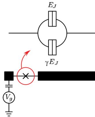
**Figure 1.** A schematic of a ‘Josephson charge qubit’. The cross denotes a *tunable* Josephson junction, which consists of two parallel tunnel junctions (upper panel). The strength of the effective Josephson coupling is tuned by flux threading the loop. The gate voltage  $V_g$  controls the induced charge on the box.
