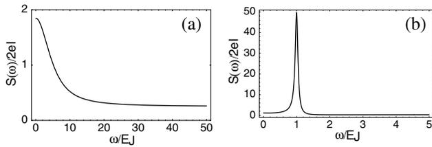
FIG. 4. Typical behavior of noise power spectrum  $S(\omega)$  as a function of frequency  $\omega$  in the (a) strong ( $\Gamma_{1,2} \gg E_J$ ) and (b) weak ( $\Gamma_{1,2} \ll E_J$ ) quasiparticle tunneling limits. For both plots,  $C_L = C_R = C_\Sigma/2$  were assumed.
